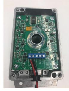
6. Secure the Altronix VR-1 unit to the duct, the air handler, or the cover of the GPS-iMeasure-D using the hook and loop tape included with the Altronix VR-1
