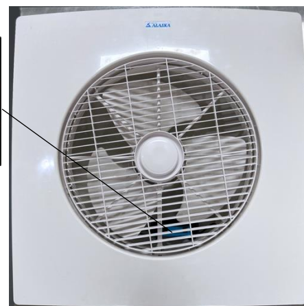
Figure 3. IDF-2 functional sample device tested with a closeup of the installed GPS's CI-2 needlepoint bipolar ionizer.
