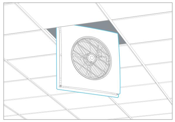
3. Slide the adjacent ceiling tile away to allow easy access to the terminal block.
