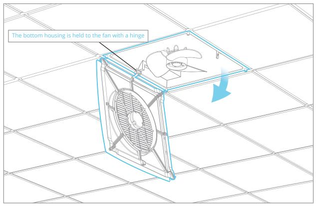
6. Reassemble in reverse order being careful to not cross thread the thumbscrews.
