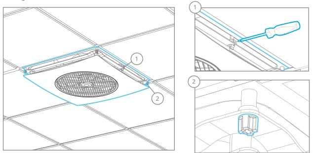
5. Once the screw and 4 thumbs screws are removed gently allow the bottom housing to rotate downwards. Use a clean cloth to wipe any visible dust and debris.
