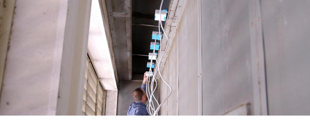
In this first test, the main variable applied was the number of Opti-Lok units powered on. The units were placed at the outdoor air intake, and the test was run using a ratio of 100% outdoor air and 0% return air. We installed a total of seven devices according to the system size, with one unit per 3,800 CFM per air source.
