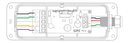
For installations in plenum spaces use only metallic clad conduit on incoming AC power. Wire colors will vary by incoming AC power and GPS product.
