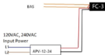
Figure 5: 120V/240V Input Power Wiring Diagram
