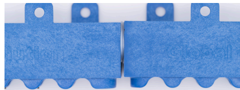
Figure 8B - Proper, small gap, filled by washer
